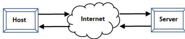
Figure 2.1: Direct Connection - The host and the server communicate directly with each other
